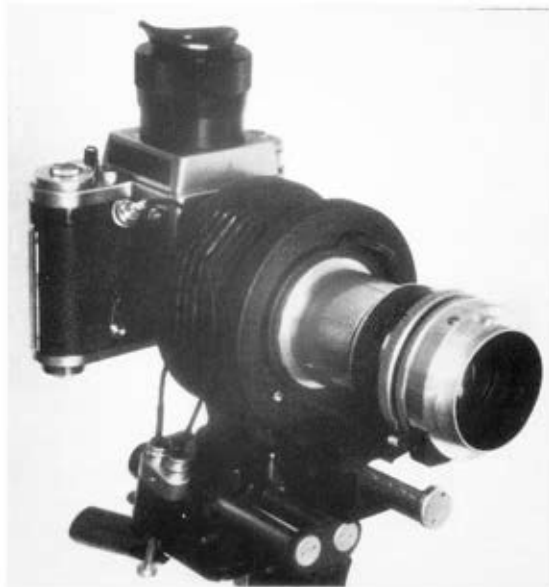
Here we can see the reversing tube in use with the bellows and double cable release connecting to the Z-ring. The metering prism has been replaced by the magnifier head.
