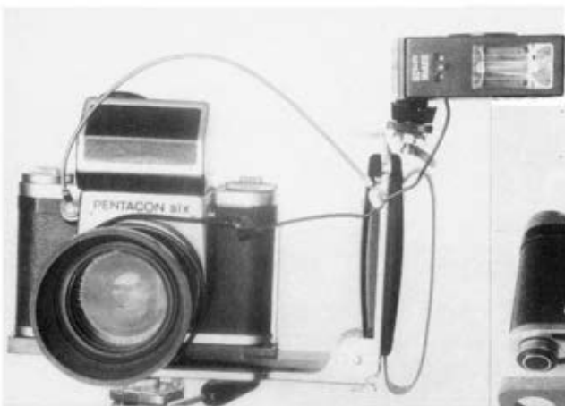
Above: The camera on a flash grip. As the knobs of the retractable spool holders protrude below the camera base, a special plate for use between the flash bracket and camera was made up by an engineer friend.
