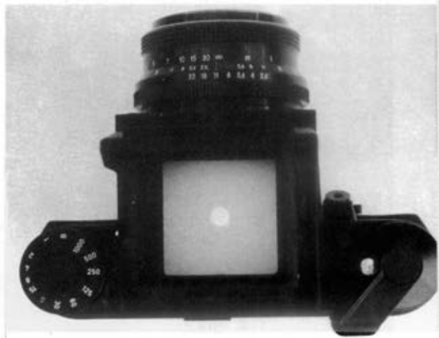
Below: The Exakta 66 top plate, showing the shutter speed dial and new index mark, and the film advance lever. A 'Mark II' version of the Exakta 66 now incorporates a very slight modification to the shape of the film advance lever, a red band on the shutter speed dial to indicate that all speeds below the flash symbol can be used with flash, and a sprung-loaded release catch for the camera back. The camera is here fitted with the Carl Zeiss Jena 80mm Biometar standard lens, which complements it perfectly.
