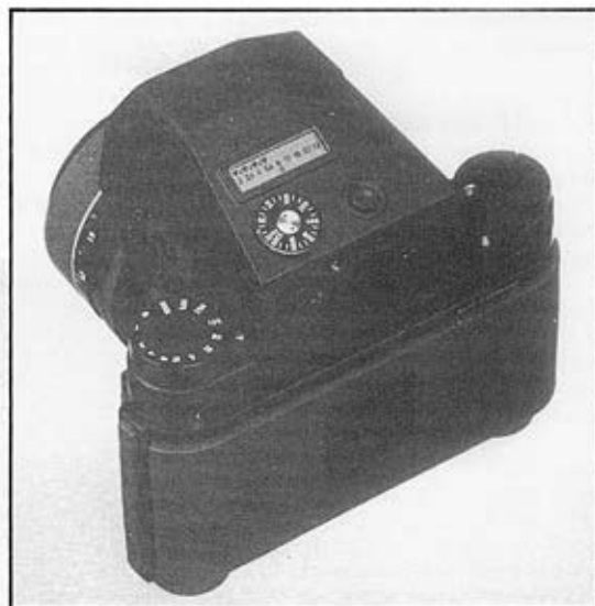
Above: Rear view of the metering prism, showing the film speed setting dial and the button that turns the meter on. The LCD readout shows that f/5.6 has been selected on the lens, and the 0 underneath the aperture numbers shows that this would give a correct exposure. Photograph courtesy of Exakta Foto GmbH, West Germany.
