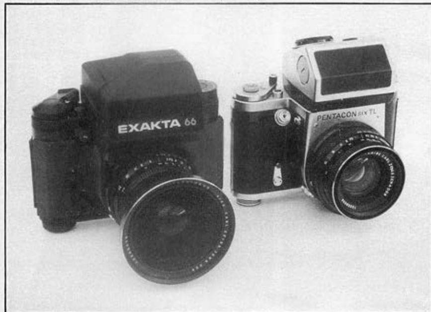
Left: The Exakta 66 and the Pentacon-Six TL, each with its own metering pentaprism. The Exakta 66 is here fitted with the outstanding 50mm Carl Zeiss Jena Flektogon wide-angle lens, while the Pentacon-Six TL has its standard lens.
